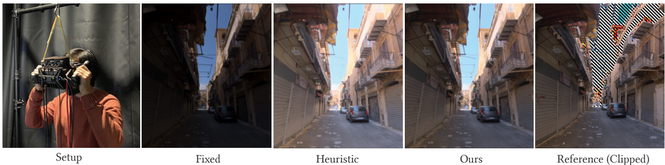
Figure 1: Three tone mapping control methods are applied to an HDR-VR scene (Section 6). While the fixed and heuristic parameter estimations fail to faithfully reproduce appearance, our method successfully finds an optimal tone-curve. Note that HDR scenes cannot be accurately represented in this document format as they were seen by our users. The rightmost image shows the unmapped HDR reference, with luminances above 100 nits clipped and marked with dashes.
